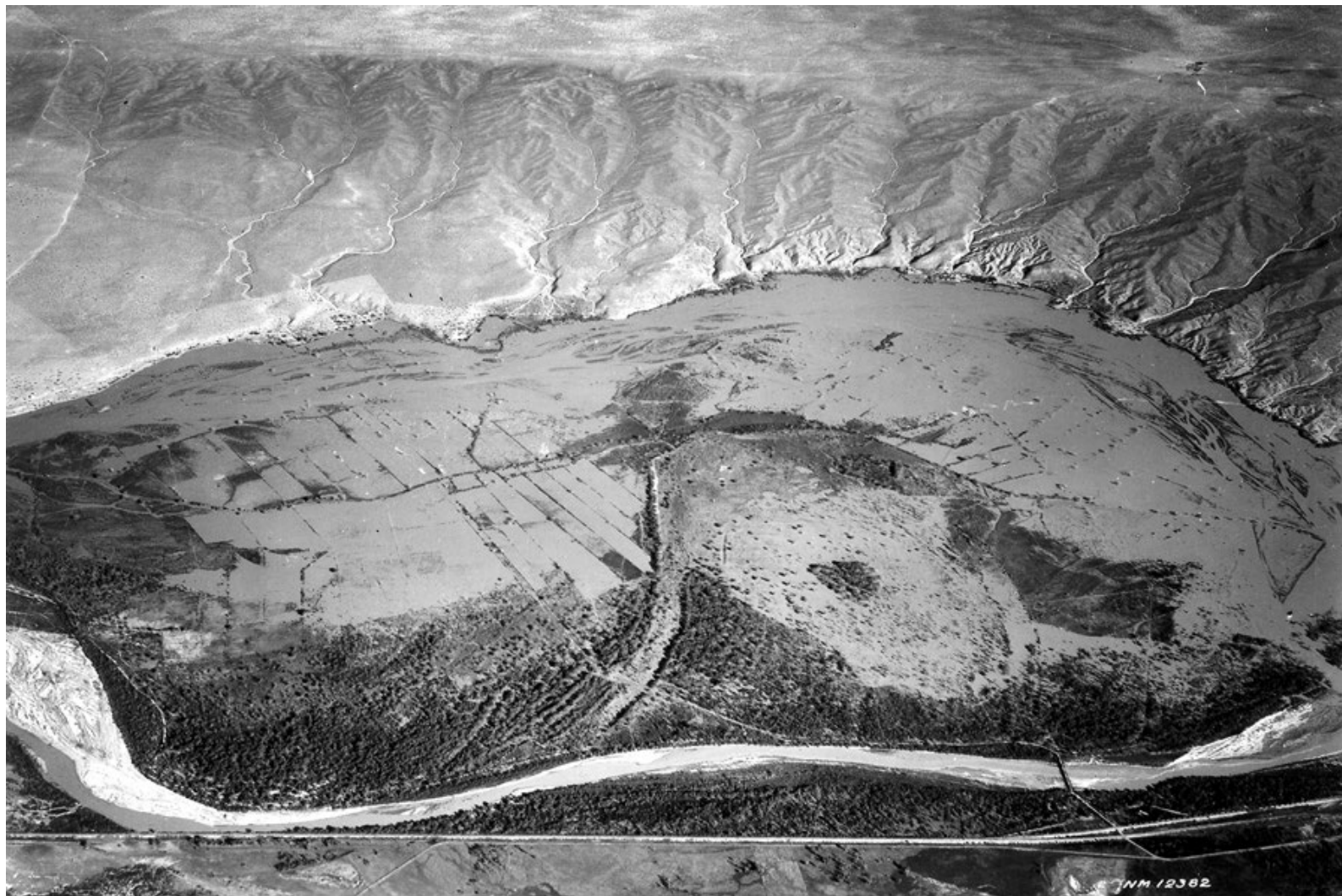
Figure 58.—Oblique aerial photo after the 1941 or 1942 flood looking southeast across Tiffany Basin with the San Marcial Railroad and the Rio Grande in the foreground (source unknown). Flow is left to right. Current channel location is in flooded area near the middle-top of photo.
