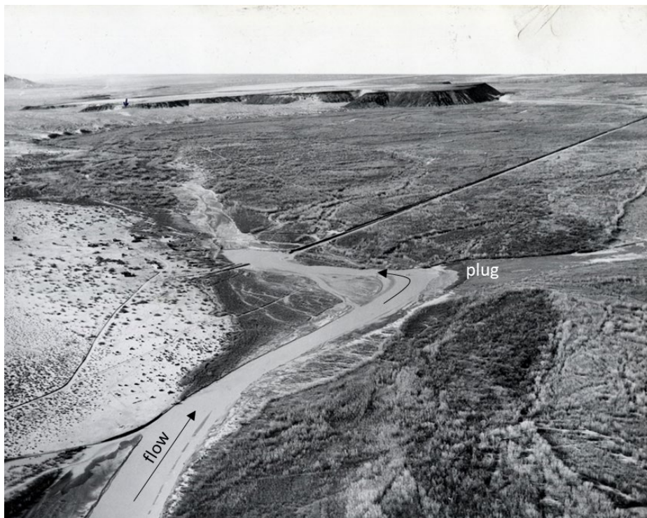
Figure 3.—Aerial photo from 1952 showing the river altering course due to the formation of a sediment plug within the San Acacia Reach above the Tiffany Basin. Low flows and dense vegetation prevented the river from cutting a new channel through the floodplain, losing surface flow connection in the upper left of the photo.
